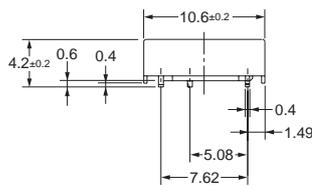
**PCB Mounting Holes (Top View)**
