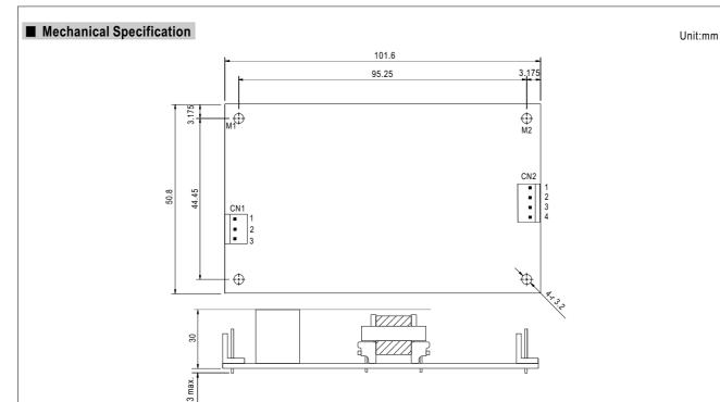
AC Input Connector (CN1): JST B3P-VH-B or equivalent
