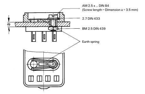
Direct mounting of relays without socket requires a fixing nut M2.5 DIN 934-m6AU. Ordering code: D00934-A0025-S001
