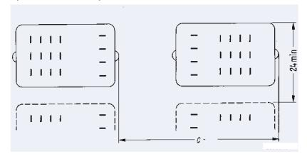
When mounting cradle relay P consideration should be given to magnetic fields. Strong DC magnetic fields, possibly caused by adjacent relays, and large iron masses are the most common causes of interference. Experience has shown that under normal operating conditions the minimum spacings specified for cradle relay P are sufficient to prevent cross interference.
