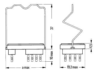
with hold-down spring for cradle relay W
